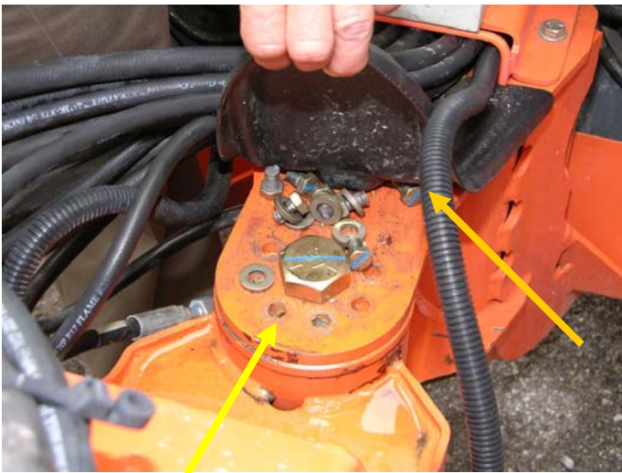
* Picture shows the sheared bolts under plate
