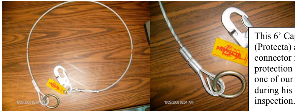
Capital Safety (Protecta) 6' wire rope cable for fall protection anchorage
