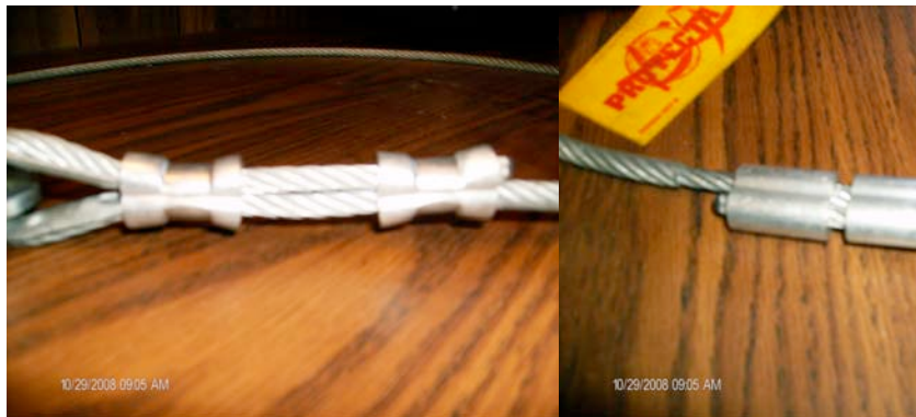
Properly crimped fittings at one end. Fittings at other end not crimped.
